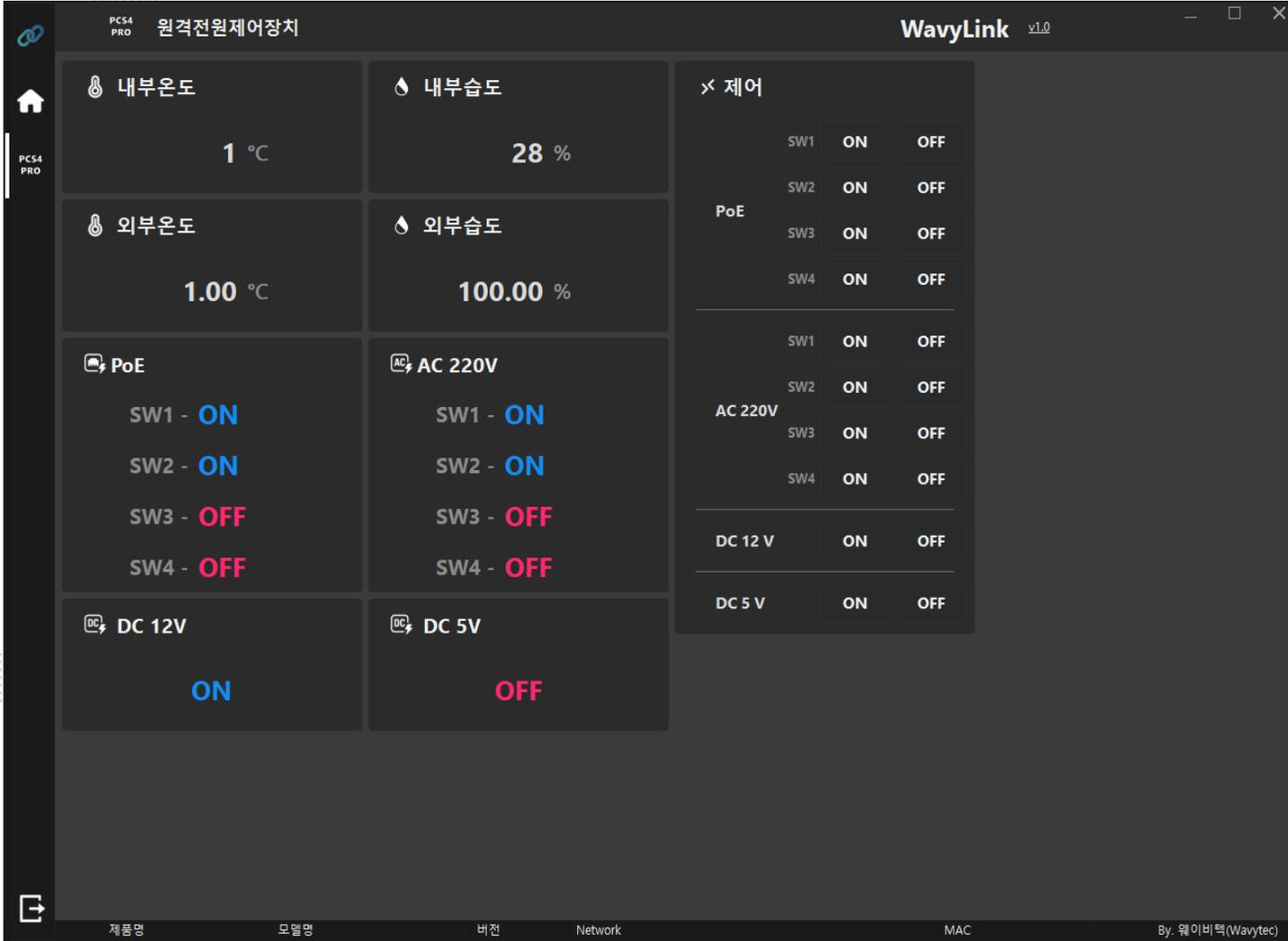
The screenshot shows the WavyLink v1.0 interface for a PCS4-PRO device. The interface is organized into several sections:
