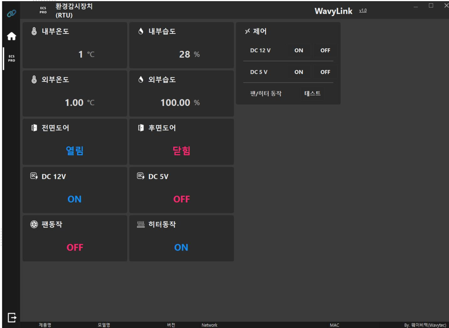
The screenshot displays the WavyLink v1.0 interface for an ECS PRO (RTU) environmental monitoring station. The interface is organized into several sections:
