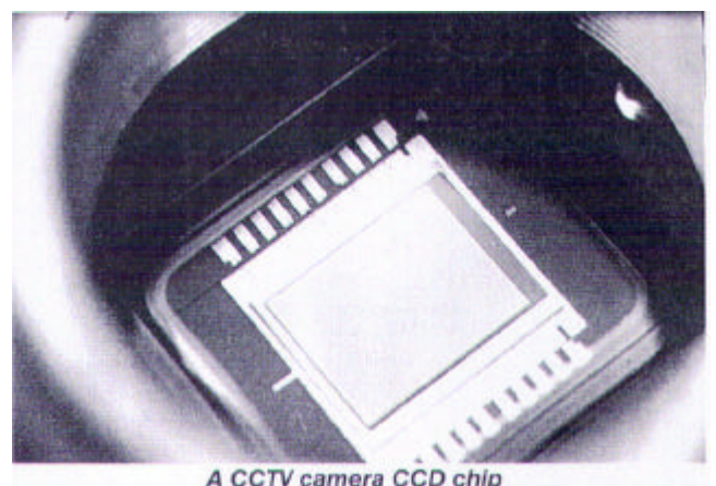
A CCTV camera CCD chip
