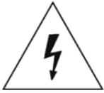
This lightning flash with arrowhead symbol is intended to alert the user to the presence of un-insulated "dangerous voltage" within the product's enclosure that may be of sufficient magnitude to constitute a risk of electric shock to persons.
