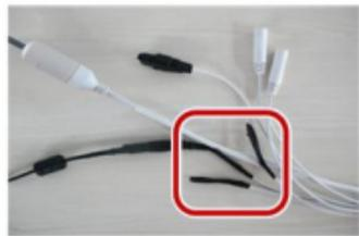
1. Connect the tail cables, and protect the cables and cable connections using insulating tapes. Then wrap all the tail cables together using insulating tapes.
