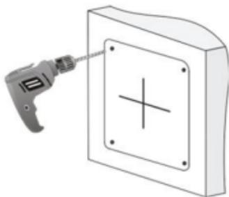
3. Knock the plastic anchors of self-tapping screws into the guide holes and ensure that they are tightened up.
