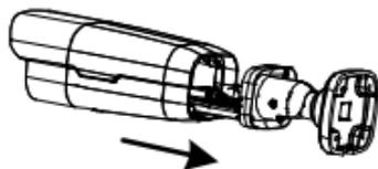
3. Insert the Micro SD card as shown in the figure below.
